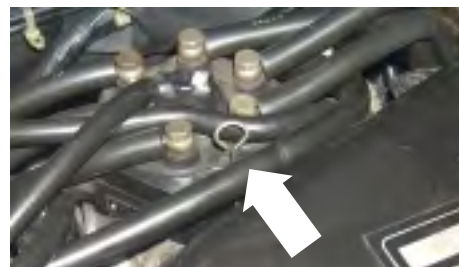
Figure 60: Unacceptable Adjuster Plug
